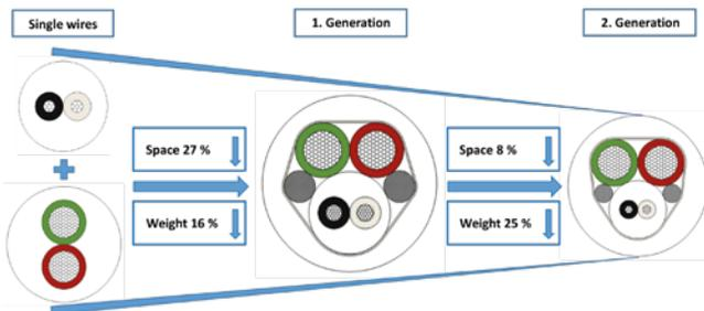
Excellent mechanical properties in terms of flex, torsion and abrasion go without saying for these types of cable because they are usually fitted along the axle. The cables must furthermore also withstand the effects of ambient conditions. As is usual with axle wiring, thermoplastic polyurethane (TPE-U) is used as the jacket material. This highly effective material is very well suited for this
