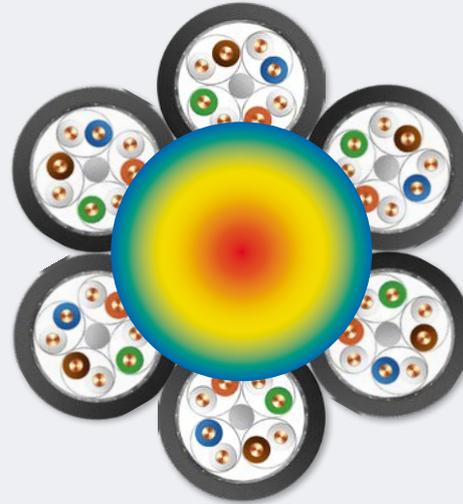
Example of application for an Ethernet cable bundle with PoE use with resulting heat generation
